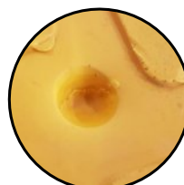
Test Results at 15°C Hammer Dropped at 3.8m
